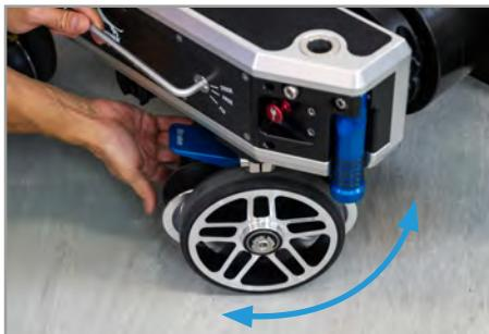
To do so you have to switch first to „FREE“ (to be able to manually move them), but after aligning switch them back to „Steer“.
