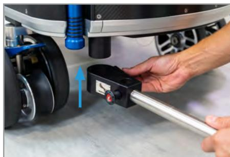
Mount the Counter Balance Rod tool-free and fasten the lever on the side to prevent an unintentional tilting of the dolly.
