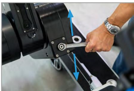
Now you can manually move the arm upwards and downwards by using the wrench.
