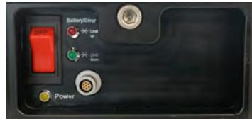
Battery empty/error: **red LED** is blinking if a maximum limit is active. It will light up when batteries are empty or in case of an error. The error can be determined by removing the electronics cover and looking at the display on the left side of the electronics housing:
