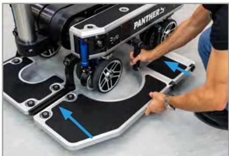
Push back the Side Platform into all holders, and the two integrated holders into the dolly.
