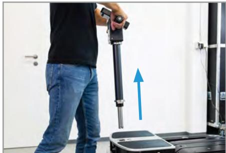
To turn it, you only have to pull it out of the dolly. Maybe you have to open the screw on the front panel with the integrated Allen Key, first.
