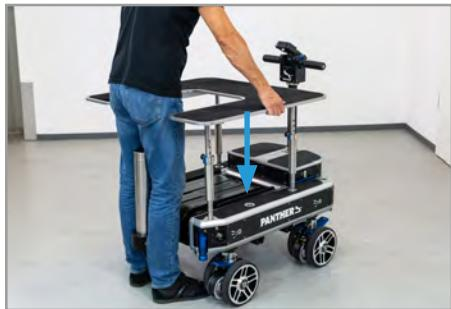
Push the High Platform's legs into the holes of the dolly (see picture on the right).
