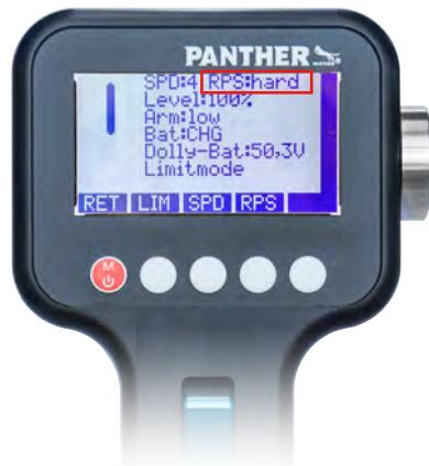
To adjust the ramps you have to **press and hold** the **RPS** button and simultaneously **tap** on the rocker (up for softer - and down for harder ramp).
