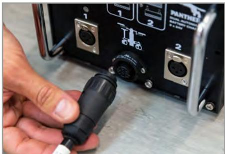
Open the protection cover of the connection socket and plug in the Power Cable (155210).
