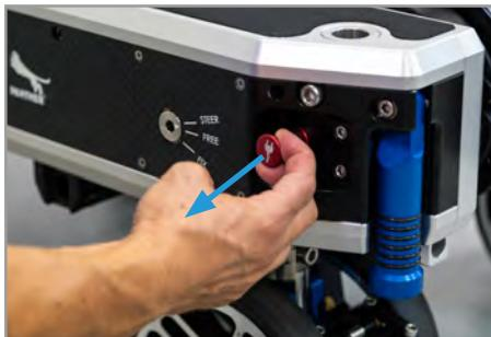
Disconnect the red electricity knob by pulling it out.
