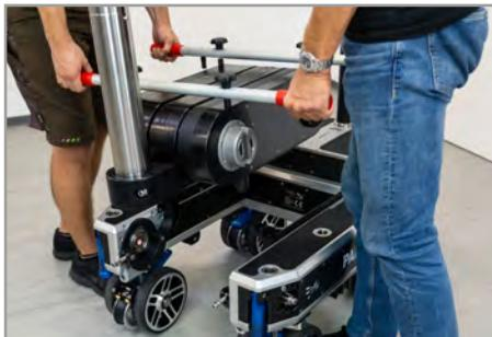
Now you need a second person. One person on each side of the dolly. You can take out the arm now by lifting both sides simultaneously.
