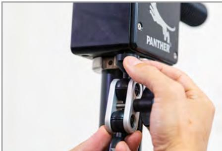
Mount the Flex Arm 3/8" on the bottom side of the S-Type Steering Rod.
