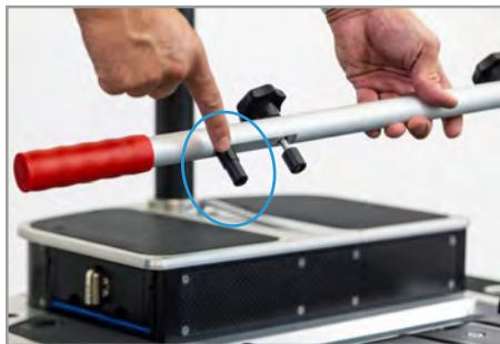
The two Carrying Rods differ in one thing: one comes with additional holders. This one is for the backside of the arm.
