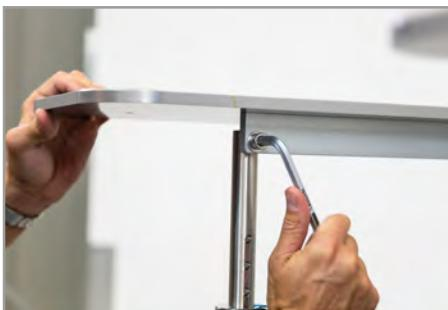
After all mountings & adjustmens make sure you tighten the screws on each leg for a safe and stable stand on the platform.
