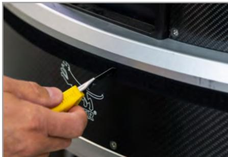
When the strip is stucked on, take a cutter and make small slits into the velcro fastener (only where the carbon cover has holes for the screws).
