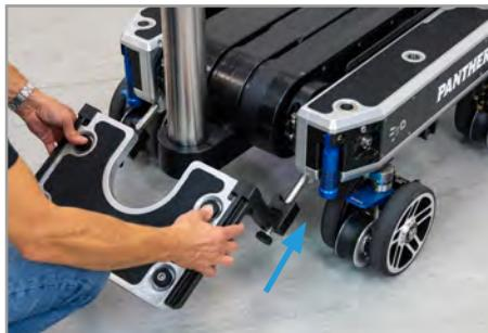
Mount the Middle Platform on the front side of the dolly by pushing it inside of the two front holes.
