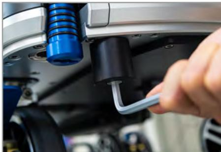
Use the integrated Allen Key to tighten the Holder.
