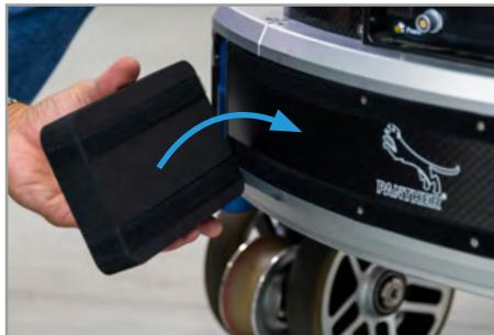
Attach the bumper to the required position along the backside of the dolly.
