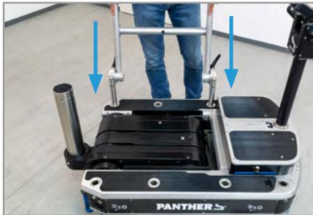
To use the Pushbar Crosswise to the track you can reposition it by plugging it in on the side of the dolly.
