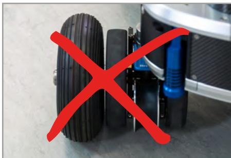
Do not mount the Big Wheels in standard gauge. Only in narrow gauge.
