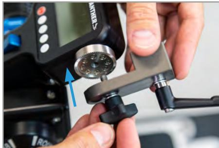
Mount the Handset Adapter 18mm to the Wireless Handset.
