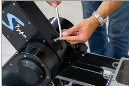
Use the integrated Allen Key to open the cover on top of the Scissors-Arm.
