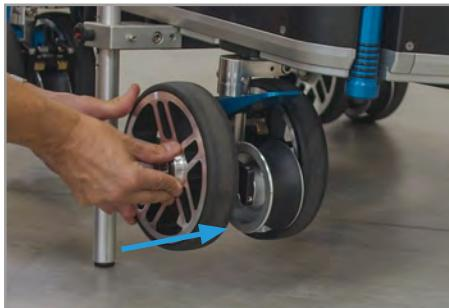
Attache the new wheel by pushing it into the Wheel Mount axis.
