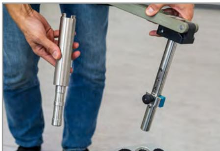
If you want to be very low, you can remove the seat arm tube by unlocking it with the blue lever and removing the tube.
