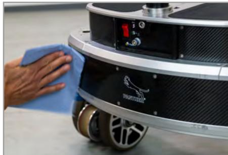
To attach the Bumper to the S-Type dolly you first have to clean the surface of the back carbon cover.
