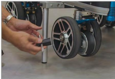
Take the Wheel Changing Tool and open the screw on the side of the wheel.
