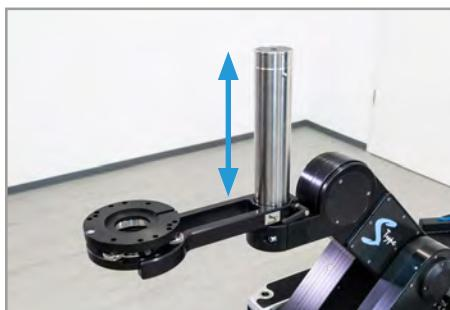
You can position the Offset Bracket everywhere along the 80mm Tube and fix it by turning the lever on the side of the bracket.
