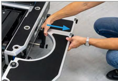
Pull the Side Platform a little bit out of the two integrated holders by holding them.
