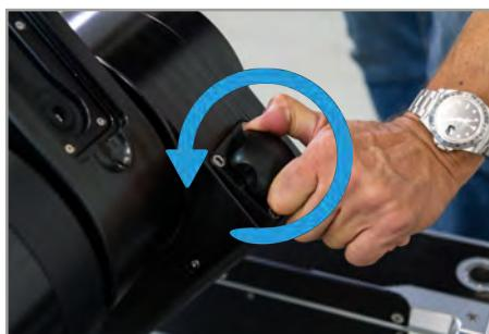
Open the cover at the side of the Scissors-Arm by turning counterclockwise.
