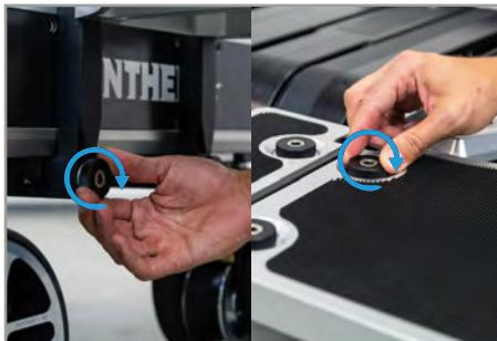
Make sure to fasten the black knobs on the Side Platform as well.
