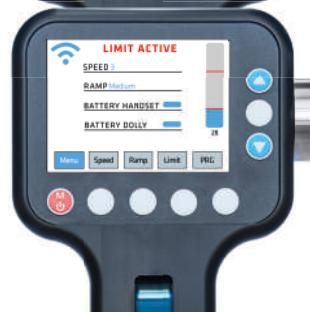
5. Back in the main menu, the limits are still indicated by red lines (or white dashed lines if deactivated). „LIMIT ACTIVE“ is also displayed in red at the top
