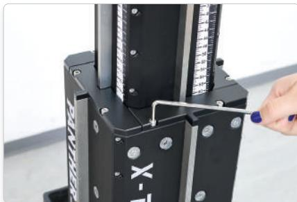
Unscrew the protective cover of the column
