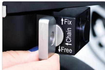
Both front wheels must be on Chain. The rear wheels must be set to Fix.
