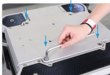
Tighten four marked screws with Panther Allen Key.
