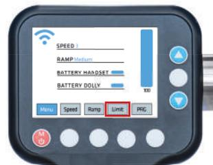
To make the up and down movements more precise, limits can be set at freely selectable heights.
