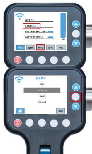
The currently set ramp of the column movement is shown at the marked position. To change this, the following must be done:
