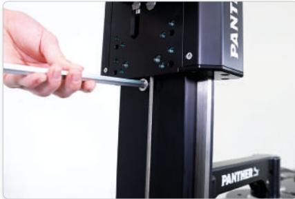
Remove the safety screw and return it to the parking position.
