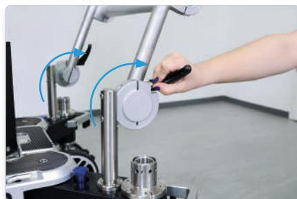
The inclination of the push bar can be customised. Release both clamping levers and lock them in the desired position.
