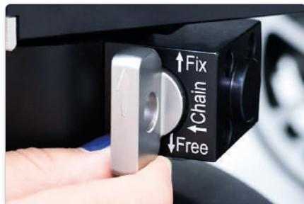
Both rear wheels must be on Chain. The front wheels must be set to Fix.
