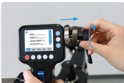
Attach the Bluetooth Handset to the handset adapter.
