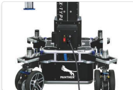
You can also charge the X-Type Dolly during use. To do this, simply connect our power cable (313426) to the plug on the front and to the charging station.
