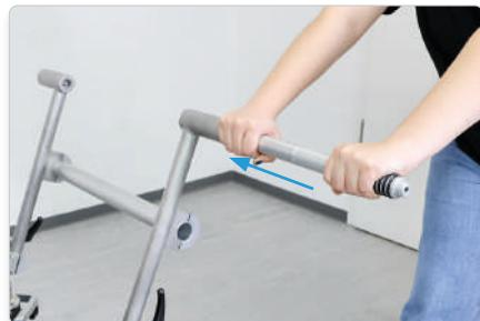
The connecting rod can also be attached to the side (on both sides) to make it easier to push the Dolly on tracks.
