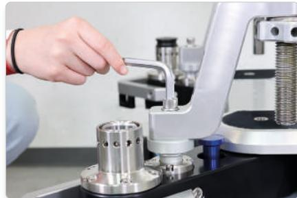
Fix the centre mount to all four wheel arms and tighten the screw shown (4x).
