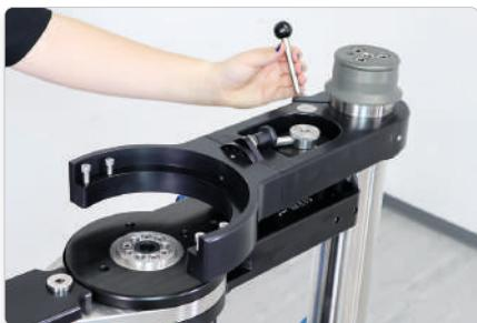
Open the lever and turn the side extension arm outwards.
