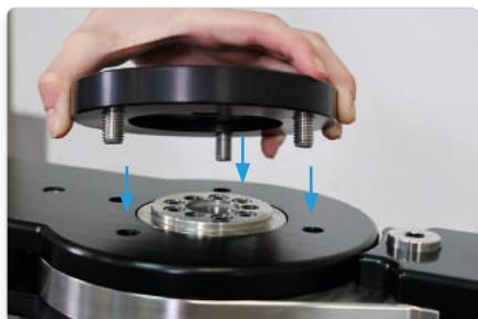
Screw the Adapter Disc to the drilling pattern on the High Low Turnstile.
