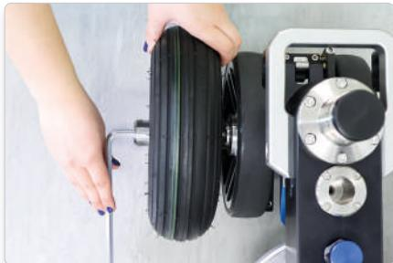
Tighten the axle from the outside with the Panther Allen Key
