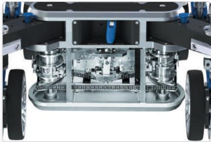
The optional Crab & Steer Kit (313494) adds the STEER mode with perfect steering geometry. This is made possible by mathematically calculated sprockets in elyptic design. The result is a low-friction, low-noise and smooth maneuvering, even in curves.
