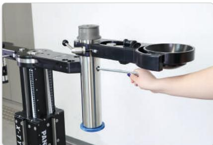
Open marked screw with Panther Allen Key.
