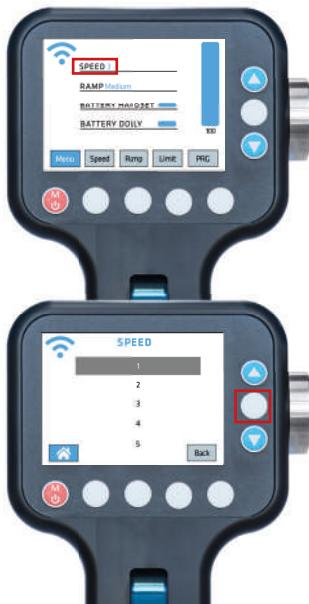
The currently set speed of the column movement is shown at the marked position. To change this, the following must be done:
