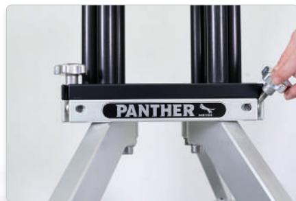
Fold up and tighten all four fixing screws.
