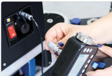
Despite charging the Bluetooth Handset on the wall socket you can connect it directly to your Dolly. Everytime you have a wired connection from the Handset to the Dolly, the Handset will be charged.
