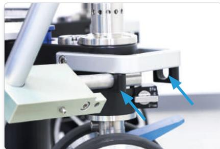
Push the bolt through the holes on the carrying handles (both holes!).
