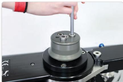
Screw the Euro Adapter onto the Adapter Disc.
