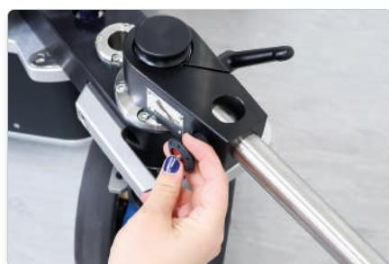
The rod can be removed by unscrewing the socket.
