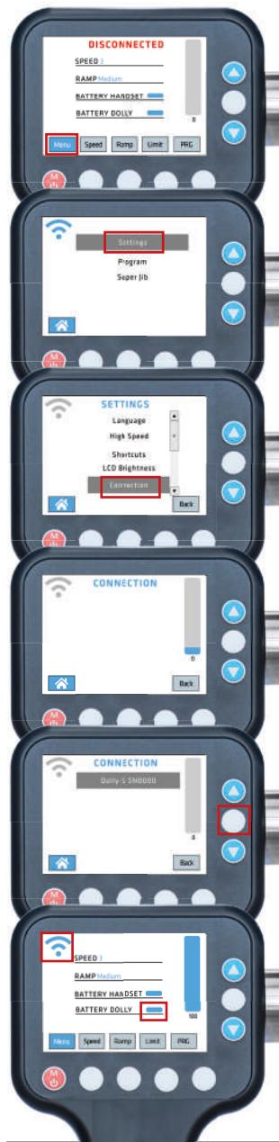
If the Handset shows „DISCONNECTED“ you need to (re)connect the Handset to the Dolly.
