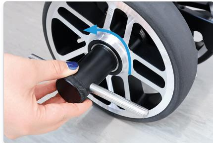
Place over the wheel nut and turn anti-clockwise.
