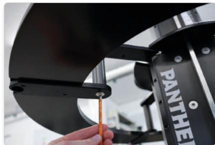
The height of the ring platform can be adjusted. To do this, unscrew four screws (M6) on the bottom.
