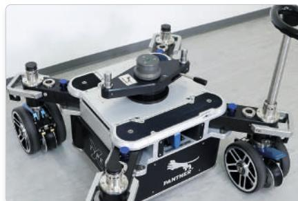
A standard drilling pattern is integrated on the base plate, on which a turnstile can be placed.
