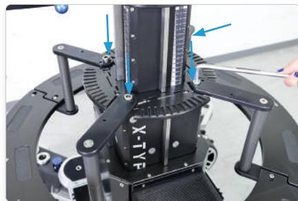
Place the Ring Platform over the Dolly and fix it using the previously removed screws.
