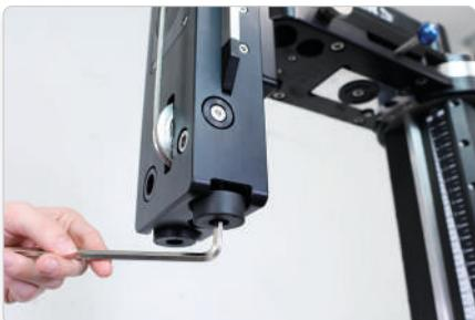
Unscrew the rubber support on the underside of the range extender.
