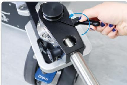
Place the Counter Balance Rod over the steering sleeve. Tighten the clamping lever.
