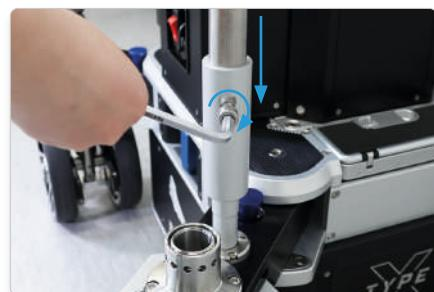
Now slide the push bar into the extension and tighten the screw shown.
