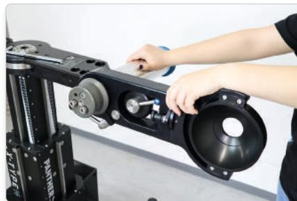
Carefully turn the pipe with the side extension arm in the desired direction.
