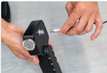
To charge the Bluetooth Handset you can use the standard charging cable (310848) and plug it into a wall socket. The display will show „charge“ instead of the remaining capacity.
