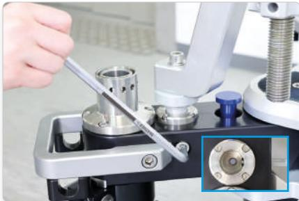
Loosen the locking screws for the holes on the wheel arms. Insert Center Mount.
