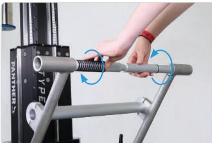
The connecting rod can be attached in the centre. To do this, attach it to one side and turn it apart.
