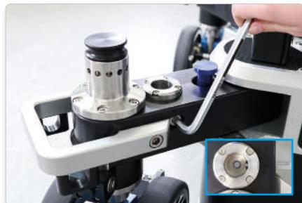
Loosen the locking screws for the holes on the wheel arms.
