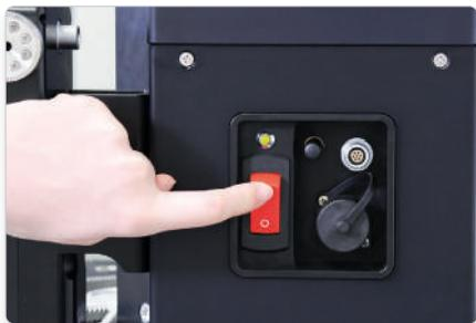
Switch the Dolly on at the red main switch. Then turn on the „On/Off“ button at the Bluetooth Handset.
