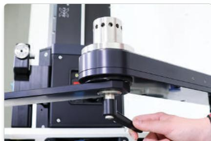
Also tighten the centre clamping lever.
