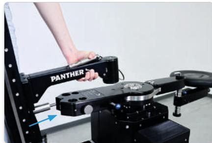
Insert Range Extender into hole of the previously detached pipe.
