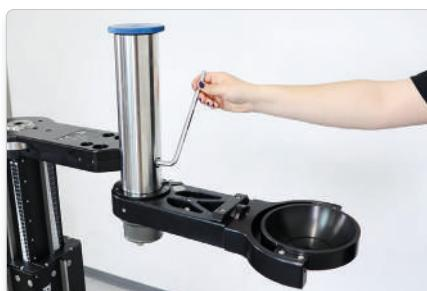
Then tighten again using the Panther Allen Key.
