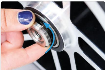
Carefully loosen the wheel nut by hand. Remove the wheel and fit the desired wheel.
