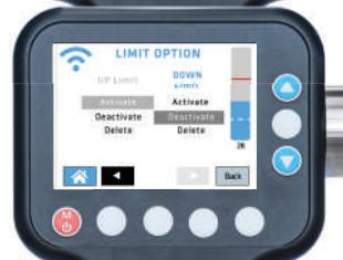
4. If a limit is deactivated, this is indicated by a white dashed line. This can be reactivated if required.
