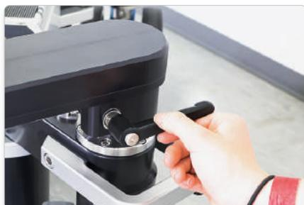
Tighten the clamping lever.
